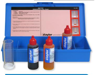
The drop-count titration in Taylor's K-1510 uses the "CAN" method (ceric oxidation of nitrite) to prevent interference in systems treated with glycol.
